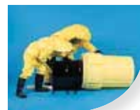
Angled rolling method can be used to manually work the drum into the overpack
